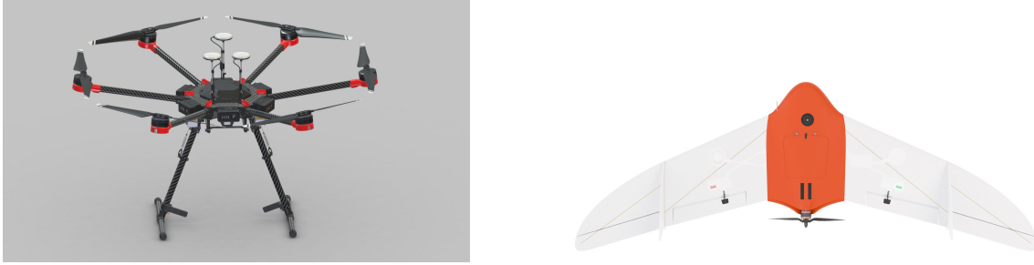
Figure 3-5: UAVs used for data collection (photos from vendor websites). Left: DJI Matrice 600 Pro that was used for the LiDAR survey. Right: Geoscan 201 Geodesy that was used for the orthophoto survey.
